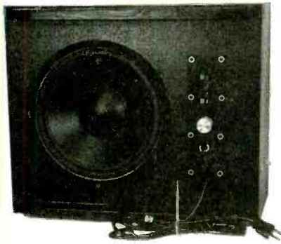
FIG. 8— CUT A 9-INCH DIAMETER HOLE in the bottom panel for the speaker and make a 7- × 1½-inch cutout for the control panel. Rails formed from 1- × 2-inch furring strips are glued to the bottom panel to hold the subwoofer above the floor.
