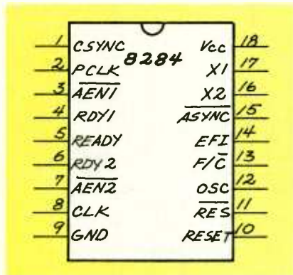
FIG. 2—THE 8284 CLOCK CONTROLLER will produce clock signals that are exactly tailored to driving the 8088.
